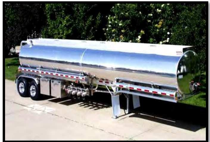
Fuel Trailer with bulkheads can carry different grades of fuel
