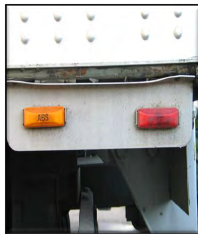
Figure 6.7 – ABS Test Light. The Amber Light will come on and stay on if there is a problem with the ABS System
